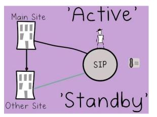
Alternatively, SIP Trunks are not just for multi-site companies. Your calls can be delivered to the same site on a separate network and on different channels.
